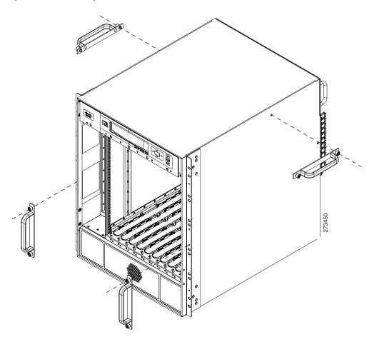
After the chassis rack-mount brackets are installed, additional handles can be installed onto the front of the rack-mount brackets. The rack-mount brackets allow a low and high installation of the handles onto the bracket depending on the chassis installation (low or high in the rack).
